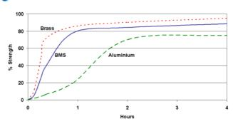
Cure times are typical at 23°C. Copper and its alloys will follow the faster cure while oxidised or passivated surfaces like stainless steel will tend towards the slower curve. Lower temperatures or large gaps will tend to extend the cure time. To reduce the cure time the use of Permabond A905, or heat, can be considered.
